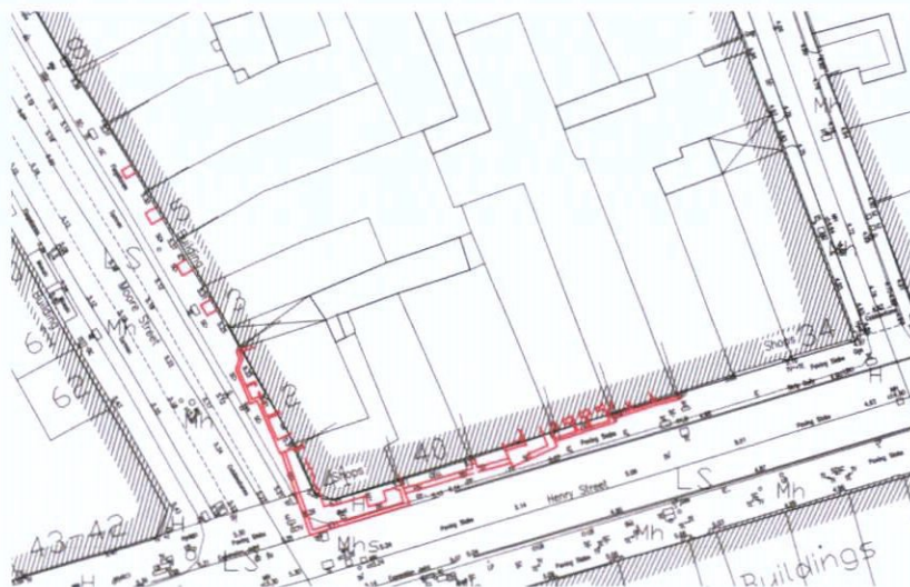
Figure 33 – Location of Existing Historical Pavement Vaults
