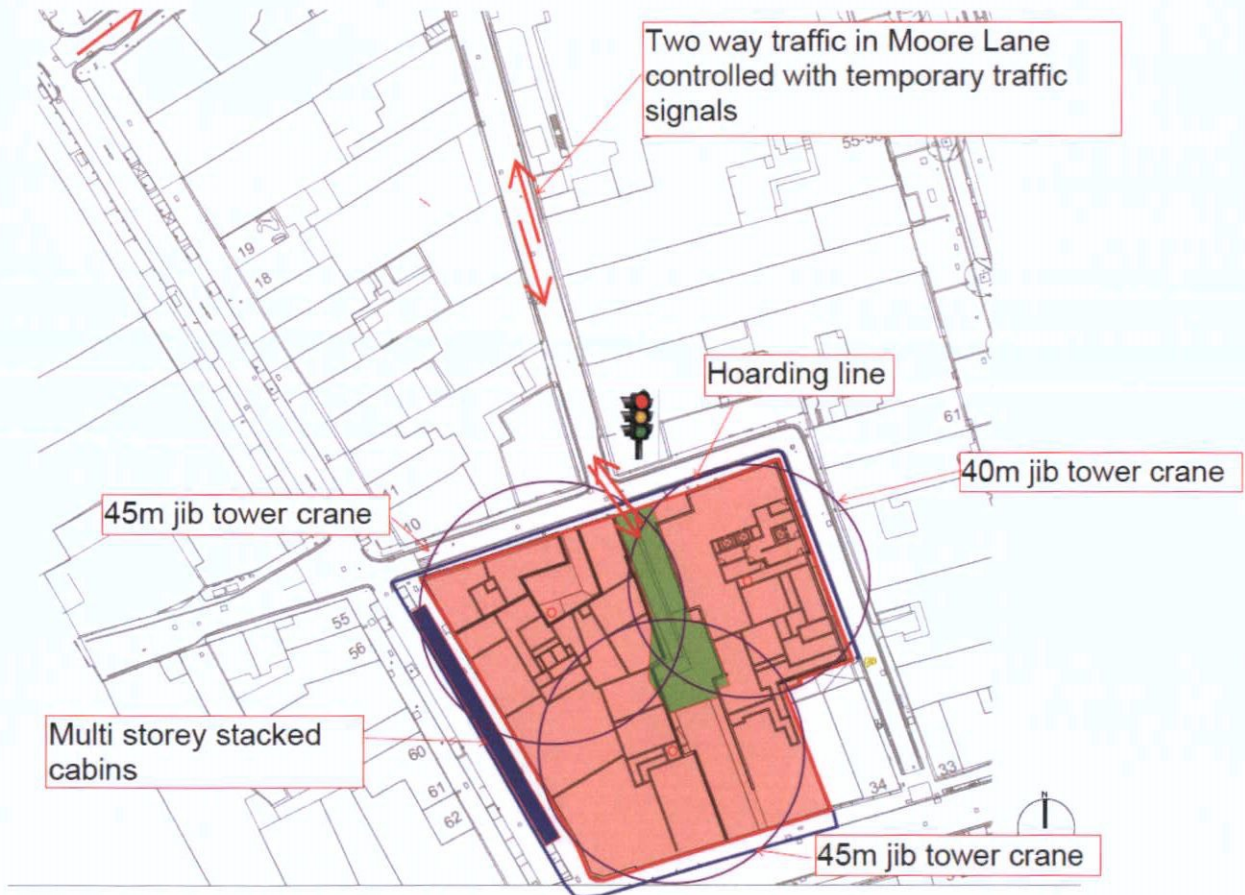
Figure 4 Site 3 Proposed Site Setup
