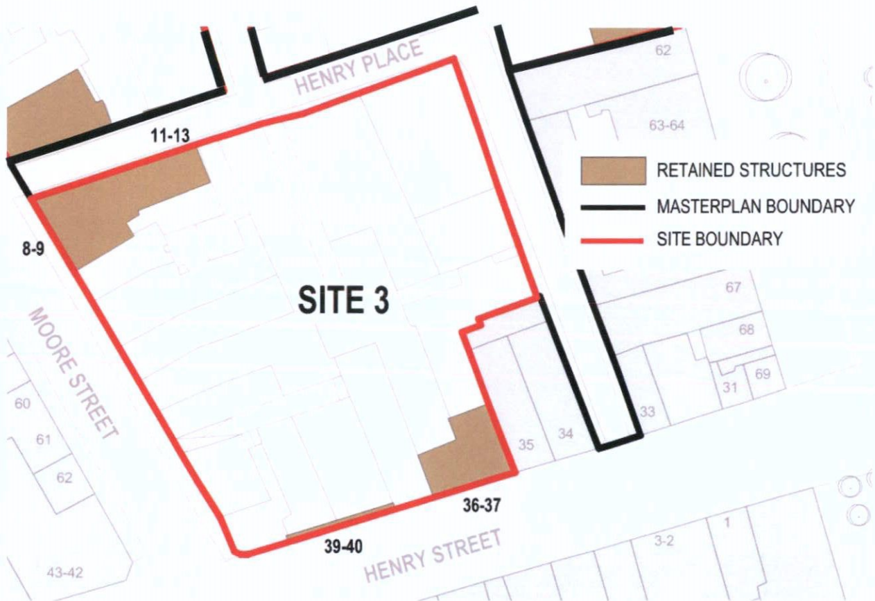
Figure 16 - Site 3 Retained Structures
